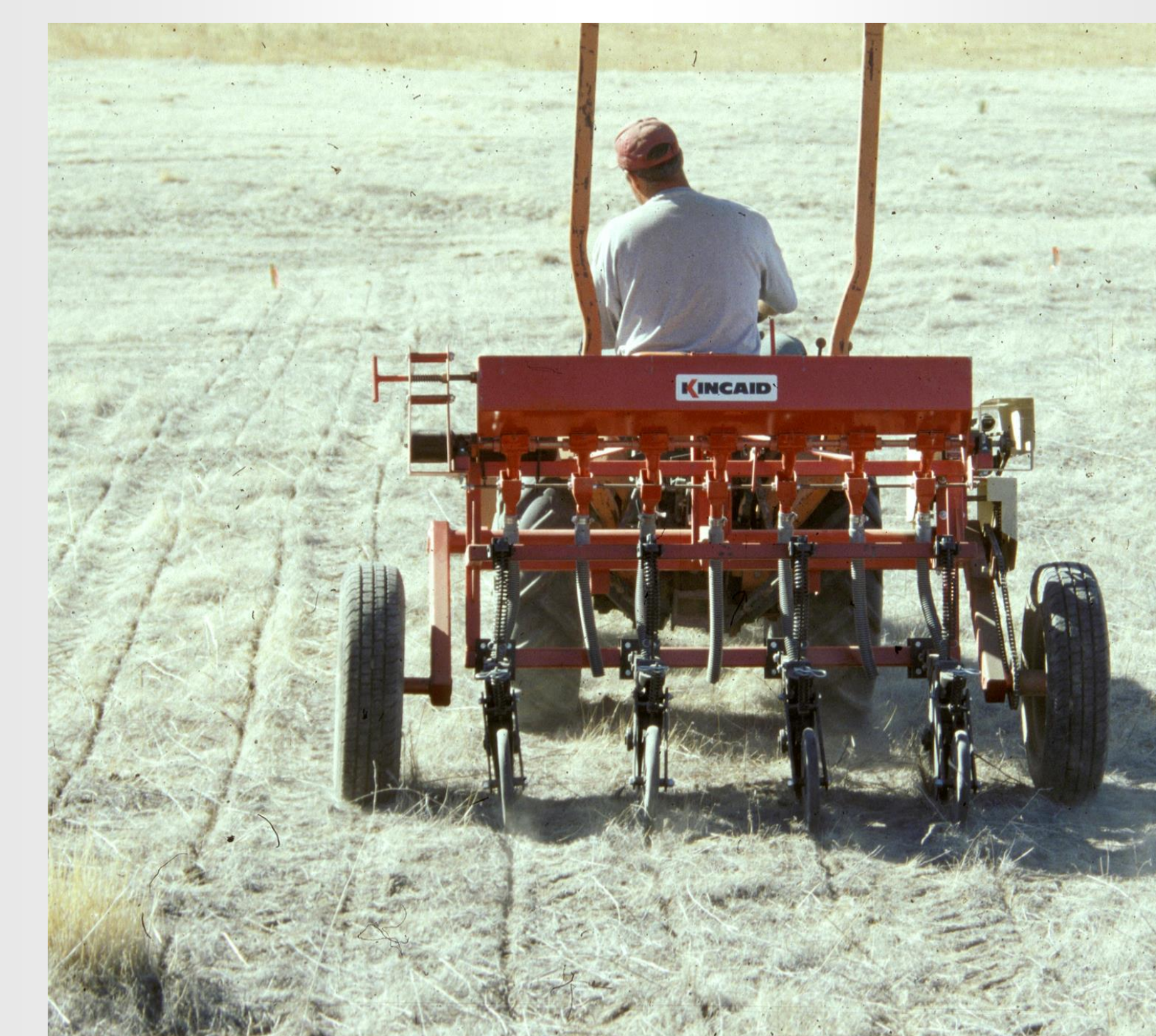
Figure 2. Seeding specific species using the kincaid no-till drill on herbicidal fallowed plot.
